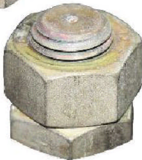
Figure 2 - Thin nut placed next to the joint.
