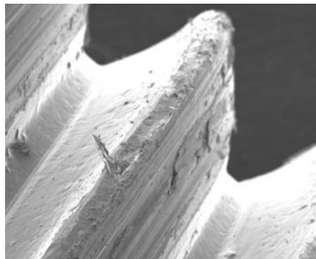
Thread surface after 10 re-tightenings
