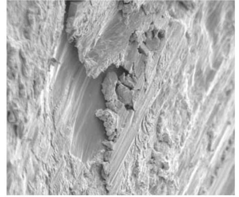
Close-up of thread surface after 5 re-tightenings
