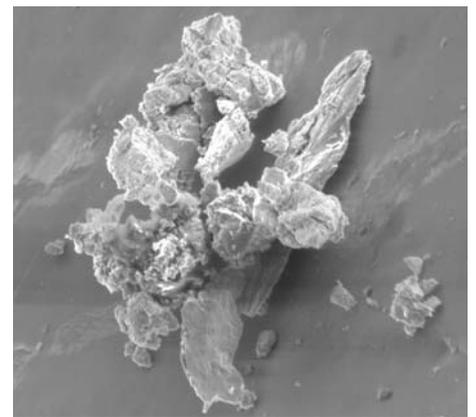
Wear particle on the thread surface 500x magnification
