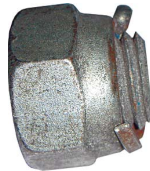
Fig. 3 — Backed-off nut resulted in the split pin being partially sheared.
