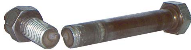
Fig. 1 — Specimen of failed bolt from bus chassis.
